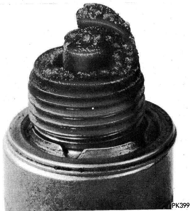
Fig. 21—Oil or Oil Ash Incrusted
