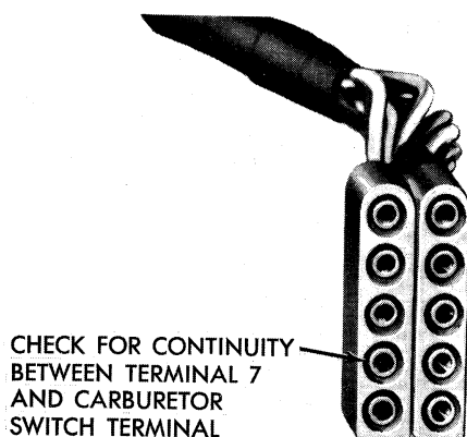
Fig. 10—Connector test (power check)
