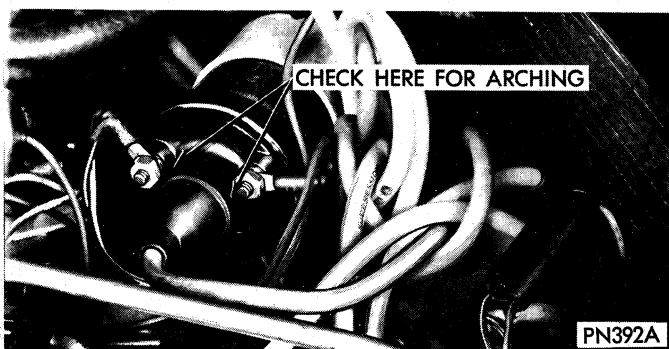
Fig. 6—Checking for Arcing at Coil Tower
