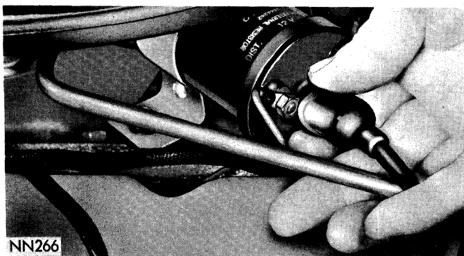
Fig. 18—Installing Secondary Cable and Nipple At Coil Tower
